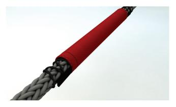
Tighten the chafe guard by using both fixing lines located in each end. The stiff eye grips in each end can be used for easy adjustment and handling of the chafe guard.
